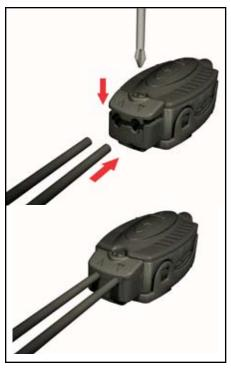
Figure 6. Installing plastic optical fiber into the FI22FP fiber ports
