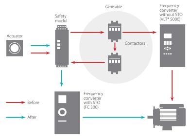
Two contactors can be omitted in safety installations due to the safety functionality in VIT® AutomationDrive
