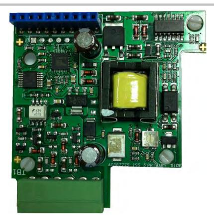
The Encoder Receiver Option allows incremental encoders to be connected directly to the motor controller to provide highly accurate speed feedback measurement. It mounts directly to the Main Control Board by means of three support stand-offs and a 10-pin interface connector built in to the board. A convenient board-mounted plug-in terminal block is provided for field connections.
