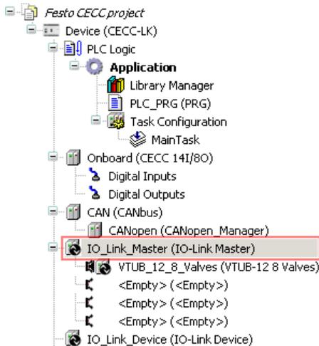
Figure: Device window - selecting "IO-Link Master"
