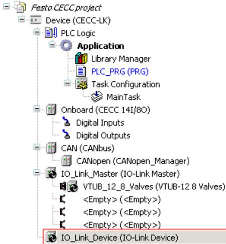
Figure: Device window - selecting "IO-Link Device"
