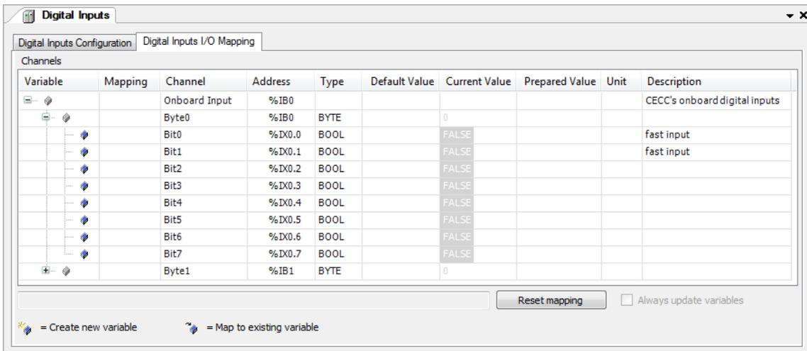
Figure: I/O mapping of the digital inputs
