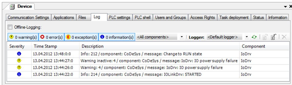
Figure: Editing window with "Device" tab - "Log" subtab
