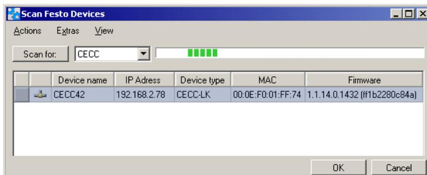
Figure: "Scan Festo Devices" scan program
