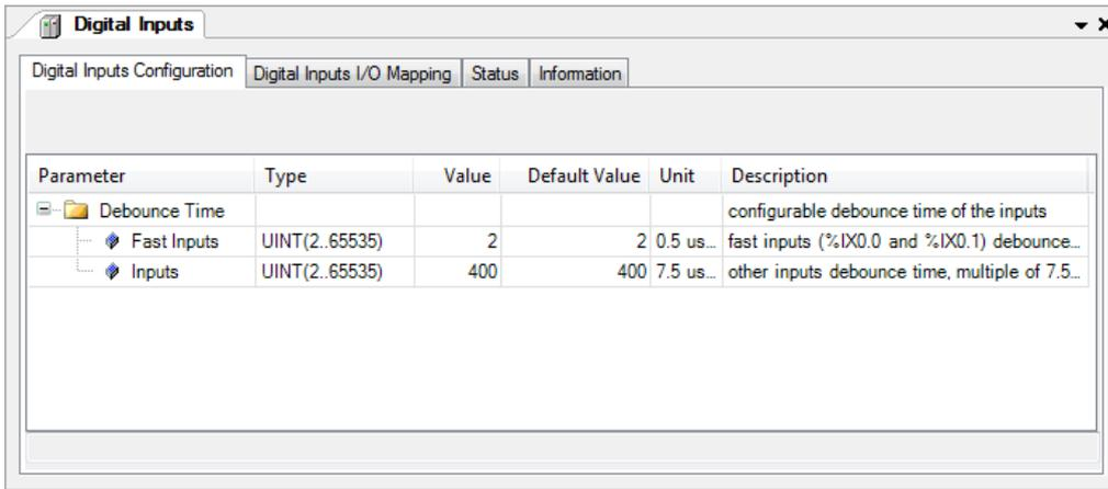
Figure: I/O configuration of the digital inputs
