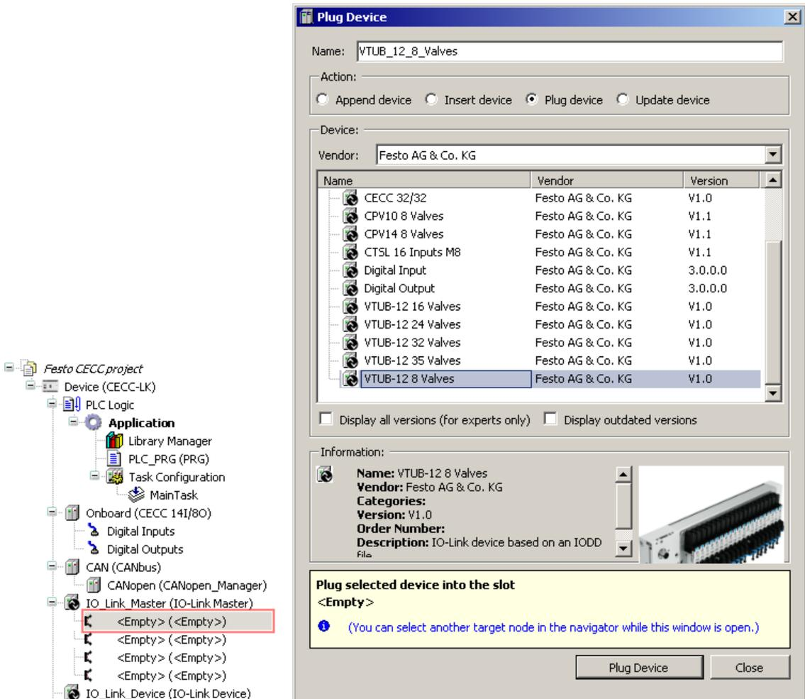
Figure: Device window - selecting a placeholder / "Plug Device" dialog
