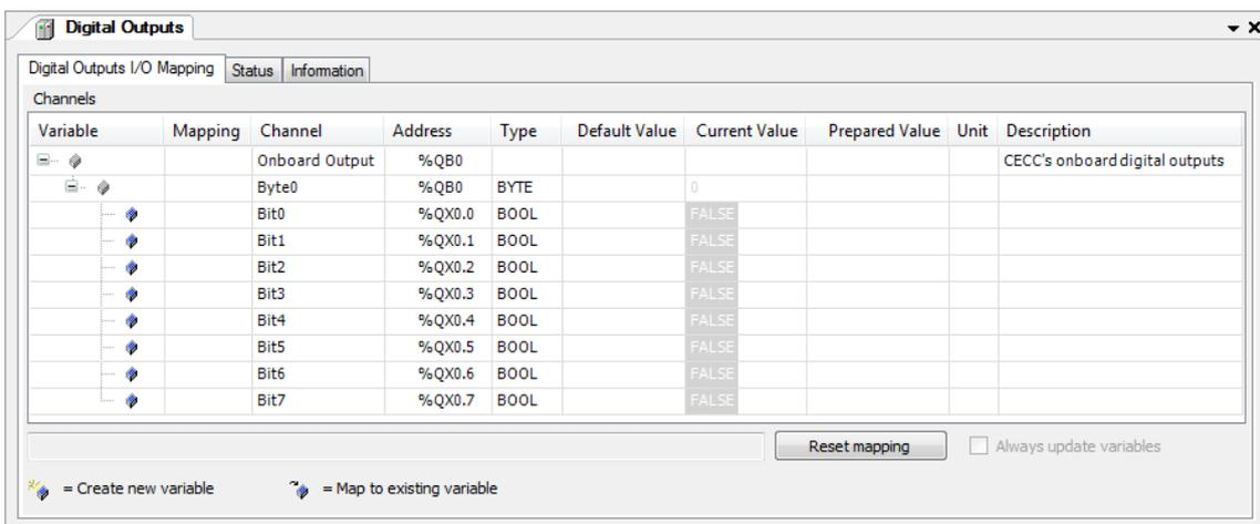
Figure: I/O mapping of the digital outputs
