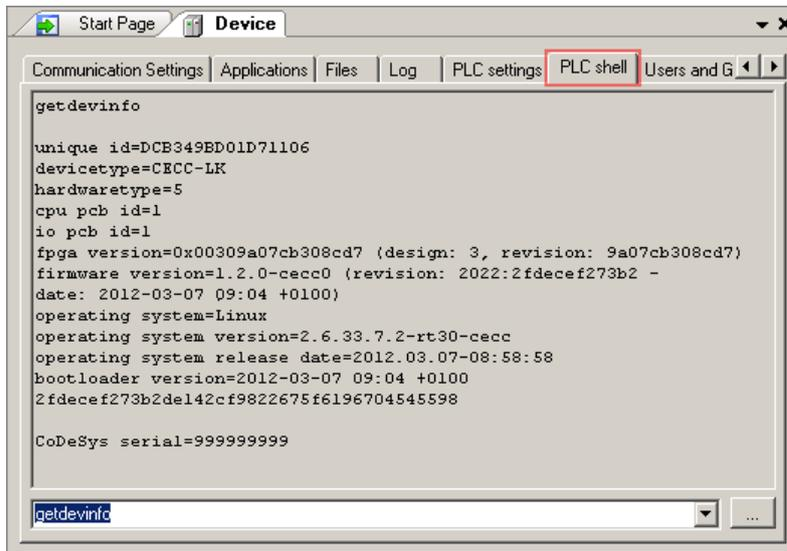
Figure: CECC editing window with "PLC shell" subtab
