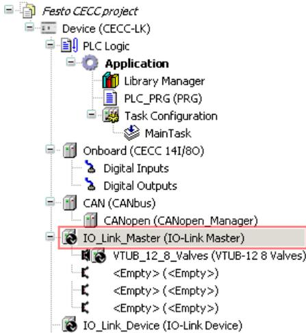
Figure: Device window - selecting "IO-Link Master"
