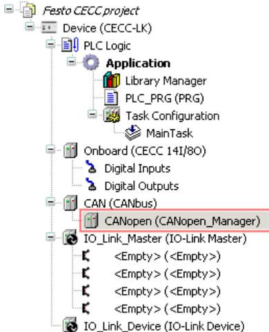
Figure: Device window - selecting "CANbus - CANopen\_Manager"
