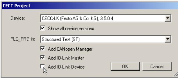
Figure: "New Project" dialog window – selecting the interfaces
