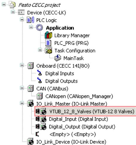
Figure: Device window - selecting an appended IO-Link device
