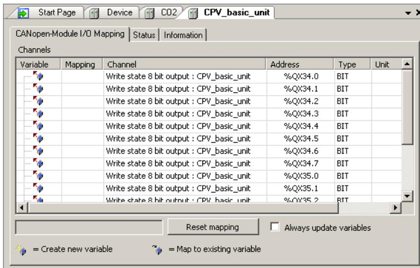
Figure: Editing window with CPV terminal as CANopen slave
