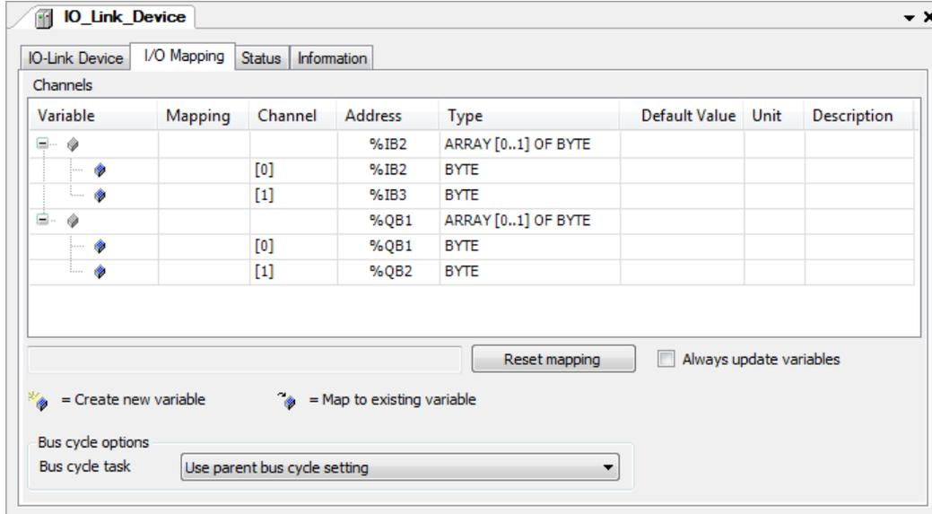
Figure: Sample onboard bus of the CECC-LK as an IO-Link device
