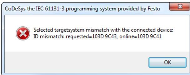
Figure: Warning message if the target system ID does not match
