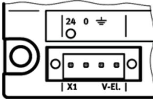
Figure: Power supply for the CECC
