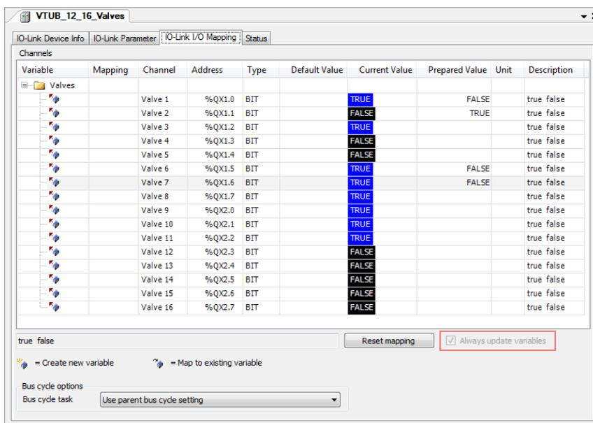
Figure: Editing window with IO-Link device "VTUB\_12\_16\_Valves"
