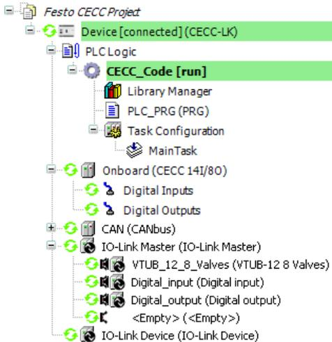
Figure: Device window with CECC in debug mode
