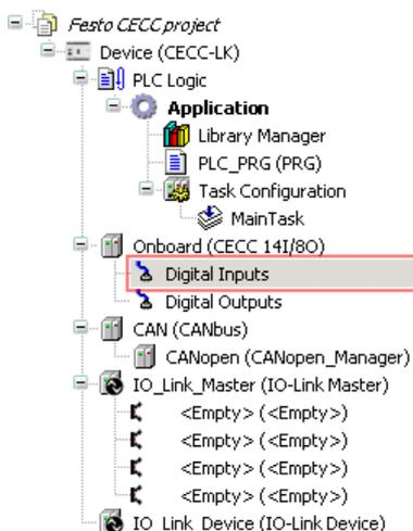
Figure: Device window - onboard I/O interface
