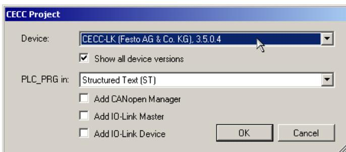
Figure: "New Project" dialog window – selecting the device
