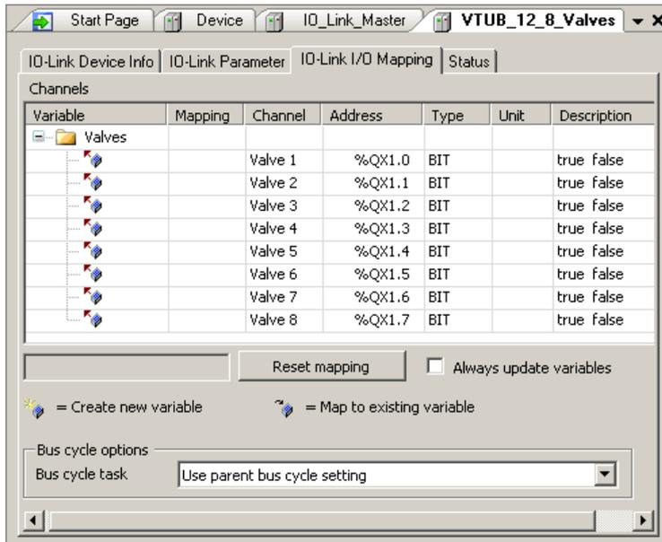
Figure: Editing window with IO-Link device VTUB-12 8 Valves (example)
