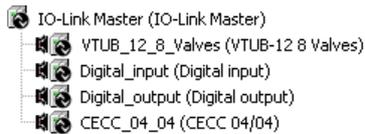
Figure: Example of an IO-Link master with four plugged IO-Link devices
