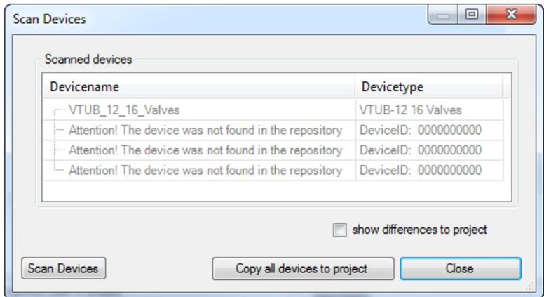
Figure: "Scan Devices" dialog window at the IO-Link masterports
