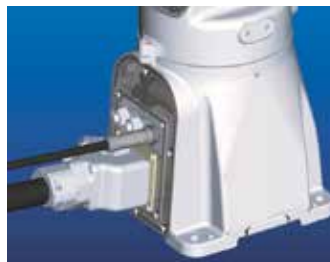
Manipulator cable connection on the side and bottom (optional) of the robot
