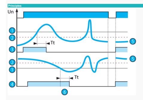
The under or overvoltage threshold value is set by a graduated potentiometer by reading the Un scale to be monitored directly. The hysteresis is set by a graduated potentiometer from 5 to 20 % of the preset threshold. The hysteresis value cannot be higher than the extremes of the measurement range.
