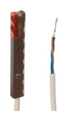
its status. 3. With the diffuse reflection sensor, the transmitter and receiver are in one device. The emitted light beam is reflected by the object that is to be detected. As soon as the receiver detects the reflected light, the switching output integrated in the device changes its status.
