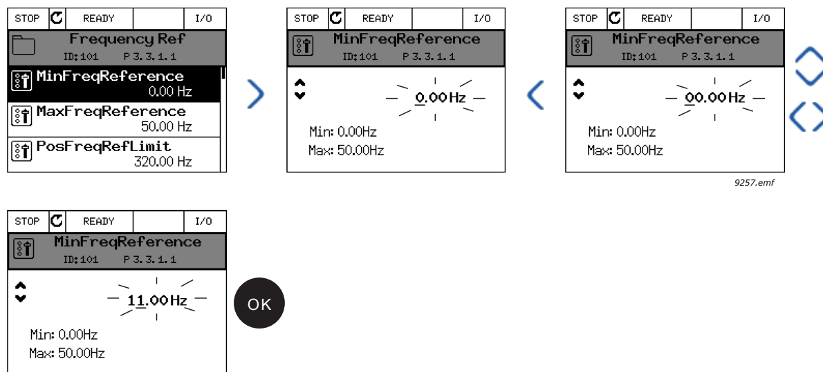
Figure 4. Typical editing of values on graphical keypad (numerical value)
