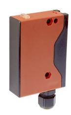
reflection sensor, the transmitter and receiver are in one device. The emitted light beam is reflected by the object that is to be detected. As soon as the receiver detects the reflected light, the switching output integrated in the device changes its status.
