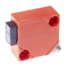
reflection sensor, the transmitter and receiver are in one device. The emitted light beam is reflected by the object that is to be detected. As soon as the receiver detects the reflected light, the switching output integrated in the device changes its status.
