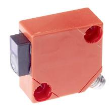
reflection sensor, the transmitter and receiver are in one device. The emitted light beam is reflected by the object that is to be detected. As soon as the receiver detects the reflected light, the switching output integrated in the device changes its status.
