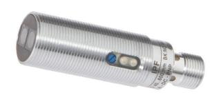
reflection sensor, the transmitter and receiver are in one device. The emitted light beam is reflected by the object that is to be detected. As soon as the receiver detects the reflected light, the switching output integrated in the device changes its status.
