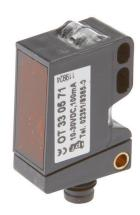
reflection sensor, the transmitter and receiver are in one device. The emitted light beam is reflected by the object that is to be detected. As soon as the receiver detects the reflected light, the switching output integrated in the device changes its status.
