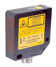
its status. 3. With the diffuse reflection sensor, the transmitter and receiver are in one device. The emitted light beam is reflected by the object that is to be detected. As soon as the receiver detects the reflected light, the switching output integrated in the device changes its status.
