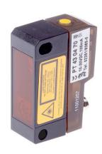
reflection sensor, the transmitter and receiver are in one device. The emitted light beam is reflected by the object that is to be detected. As soon as the receiver detects the reflected light, the switching output integrated in the device changes its status.
